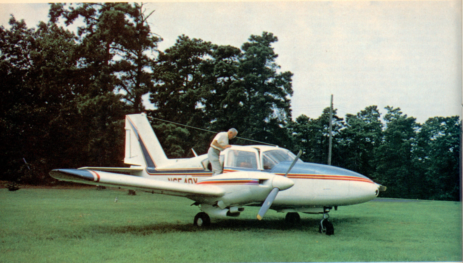
Color scheme of Aztec D is simpler and stronger than previous designs. Plane's dimensions remain same as those of previous model. Nose and rear compartments hold 150 pounds of baggage or cargo each.
